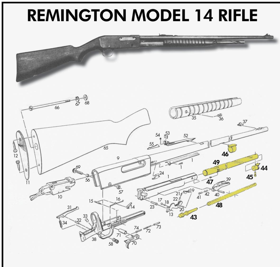
This is a schematic for the Remington Model 14. It is a pump-action rifle, first produced in 1912. The magazine parts are highlighted with color.
